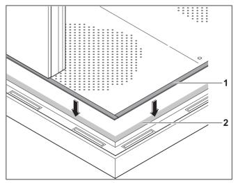
Make sure that the inner floor panel is free of grease and dust in the area of the inner wall panel (2).
