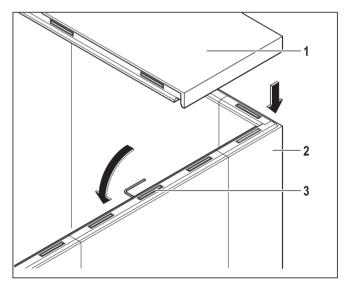
Place ceiling element (1) onto wall elements (2) and tighten eccentric cam locks (3).
