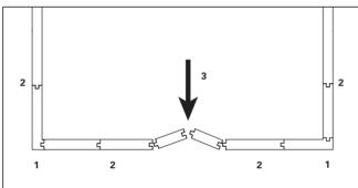
4.9 Assembling partition wall of combination rooms without tongue and groove system
