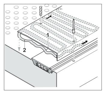
Place the stainless steel doorsill (1) in the middle between the door soffit on the floor element and align.
