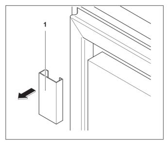
() The magnetic sealing frames on the doors are protected from mechanical damage by securing plates.
