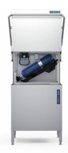
deep tank of the Metos WD-8A PPE Autostart equipment washer prevents the wash water from frothing. A deep tank together with effective filters keeps the wash water cleaner for longer. The wash pump and washing arms are self-draining prior to the final rinse, thereby preventing wash water dropping on clean equipment.
